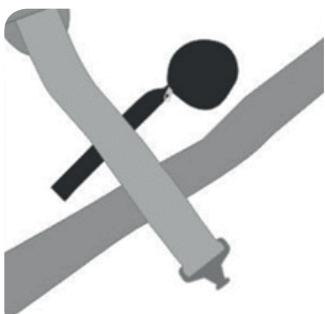
Slip the strap case through the harness loop that contains the leg strap.
